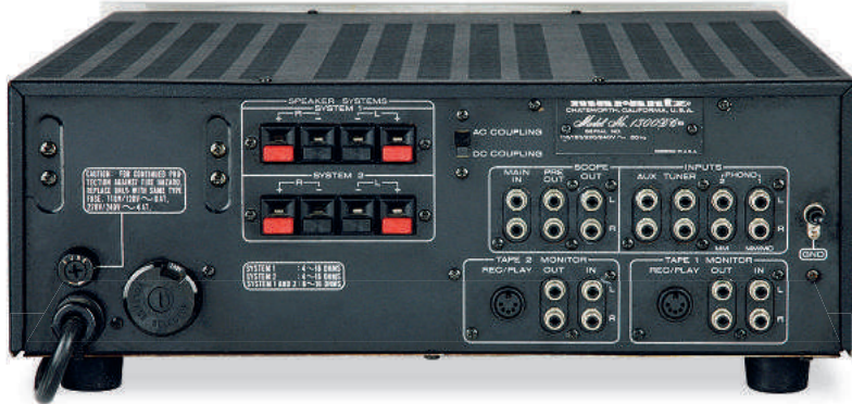
ABOVE: The rear of the amp offers a socket for everything you could possibly need. This European model has a mains voltage selector, US versions (115V) may not
